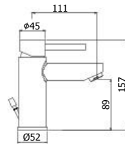
SK 071H-075HCR-EWS Miscelatore lavabo con/senza scarico, con cartuccia ENERGY & WATER SAVING Wash basin mixer with/without pop up waste, with ENERGY & WATER SAVING cartridge
